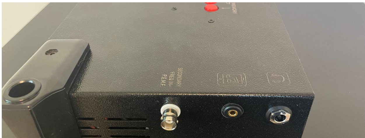
Figure 6 Right side of control box. L to R : auxillary input for PEMF, 3.5mm audio input, 1/4" headphones output
