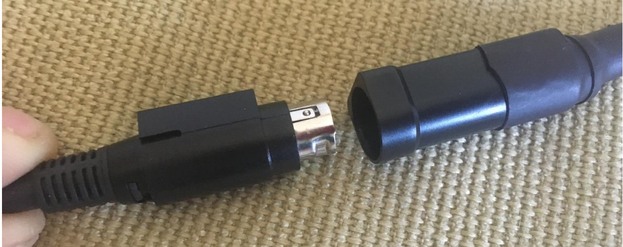
Figure 3 removal of power connection. Left side will allow removal by moving in and out
