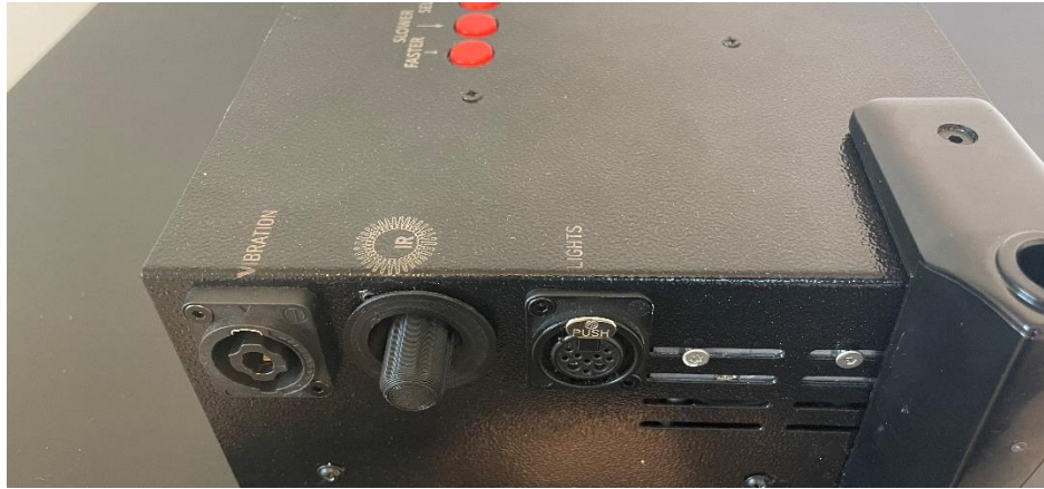
Figure 5 left side of control box. L to R : vibration, IR brightness, Lights
